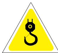
Crane in operation
